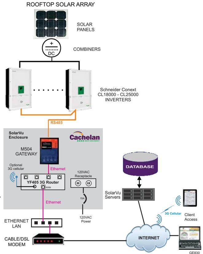
Fig 2 SolarVu Enclosure components and connection
